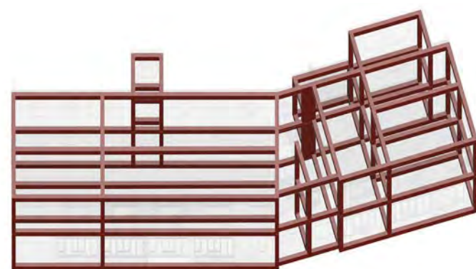
Primary Structure Reinforced Concrete (RC) Frame
