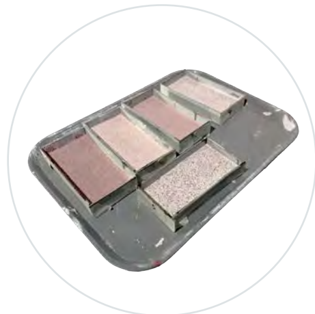
Casting the Plaster
